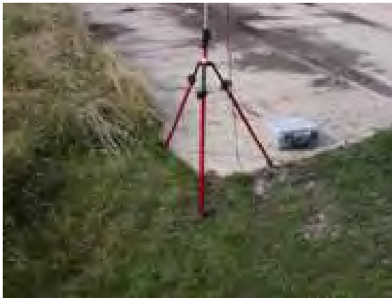
Figure 2 Picture of GCP with the rover station
