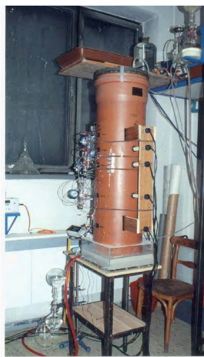
Figure 1 Experimental setup of the soil column in the laboratory and diagrammatic drawing
